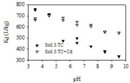
Figure 2. Effects of pH on TC sorption on Soil 3 in the presence and absence of Cd.
